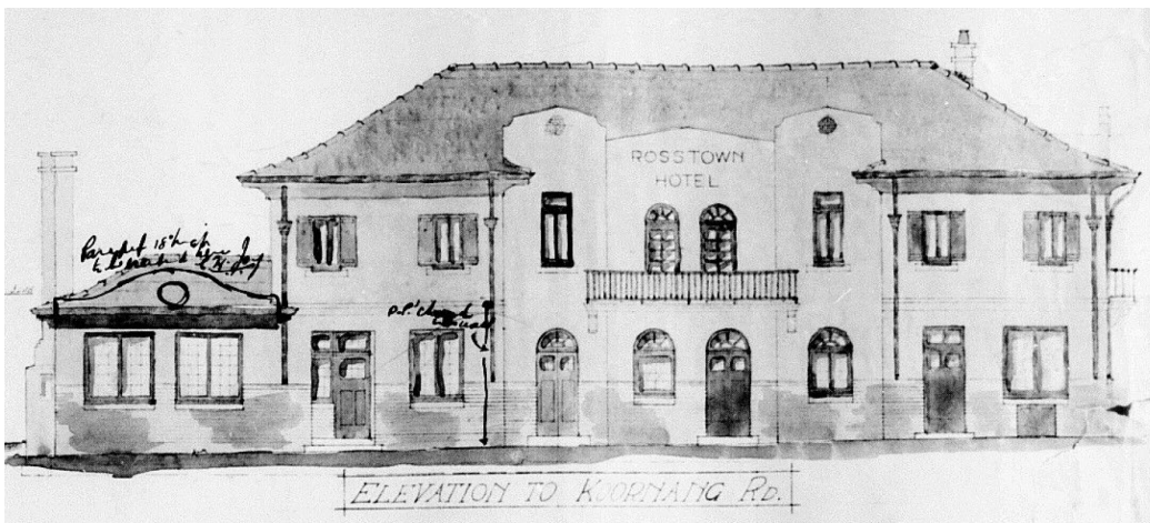
Koornang Road Elevation, date March 1926. Note the amendment introducing a parapet to the single storey portion (not reflected on other drawings such as the roof plan).
