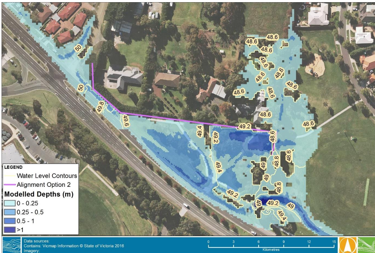
Figure 3-4 Alignment Option 2 and 1% AEP Modelled Flood Depths
